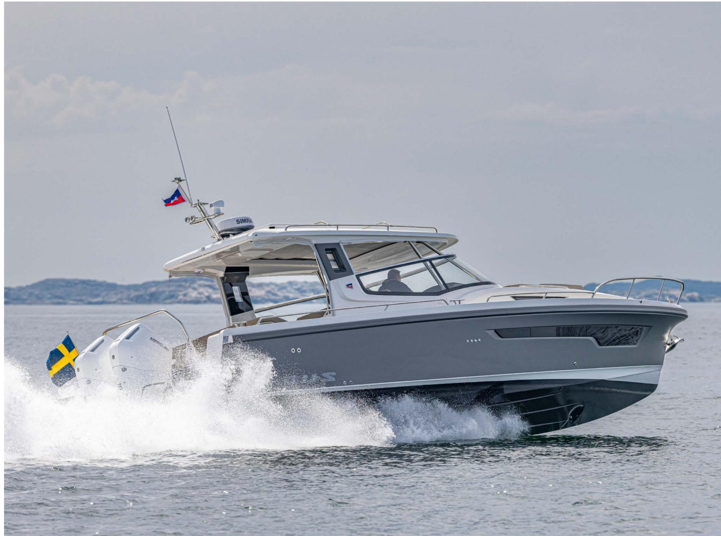
controls to operate the Quick gyro stabilizer. I start to accelerate slowly, because I want to see how snappy the W11 is with its 2 400hp Mercury Verado V10 outboards, and the response is impressive, as soon as I touch down on the throttle we are already at 12 knots, almost on glide. I accelerate harder, and after a short while I've already reached 23 knots, however, I feel like I'm floating.
